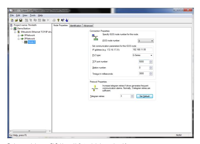
Each new node is a new PLC driver, with first node being numbered 0.
