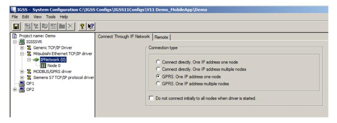
When the GPRS options are selected, you can design a schedule which the driver will use when connecting to the PLC node.
