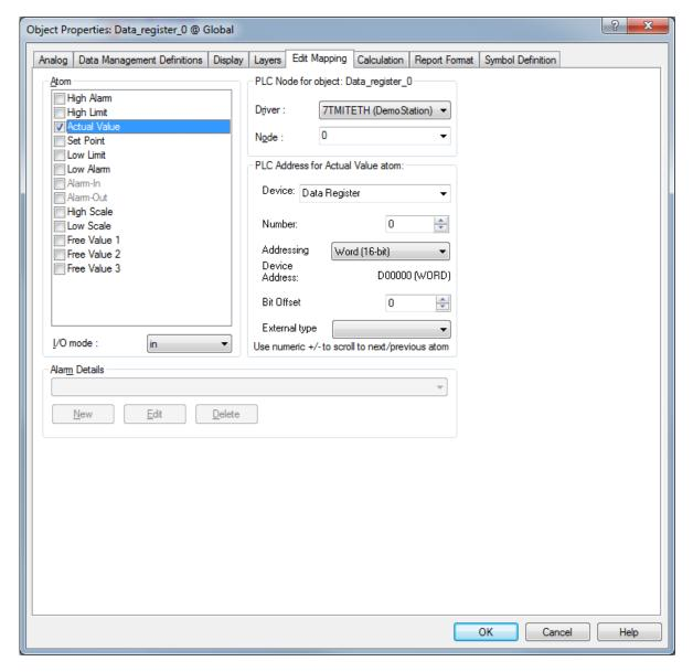
Now select the desired PLC node number and continue by setting be desired Device. Then specify the number (register number within the device type). Note that the corresponding Mnemonic is displayed and updated as you select the appropriate parameters. This is a help to make sure you always bind to the correct process variable.
